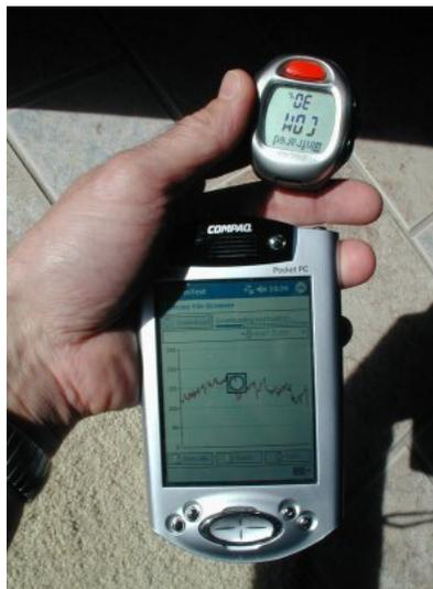
**Figure 18: Downloading workouts from a Polar S720i into a Compaq iPAQ 3970.**
